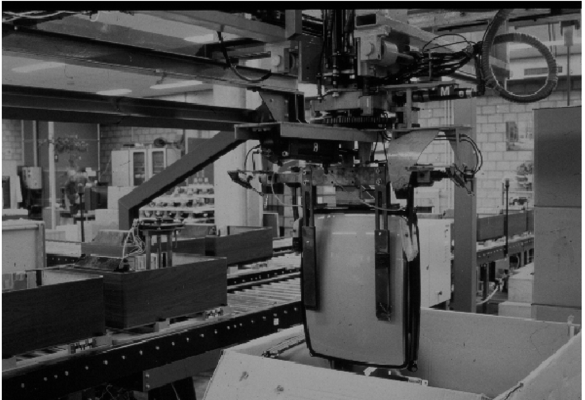
Television Set Assembly: MATS/flow production
