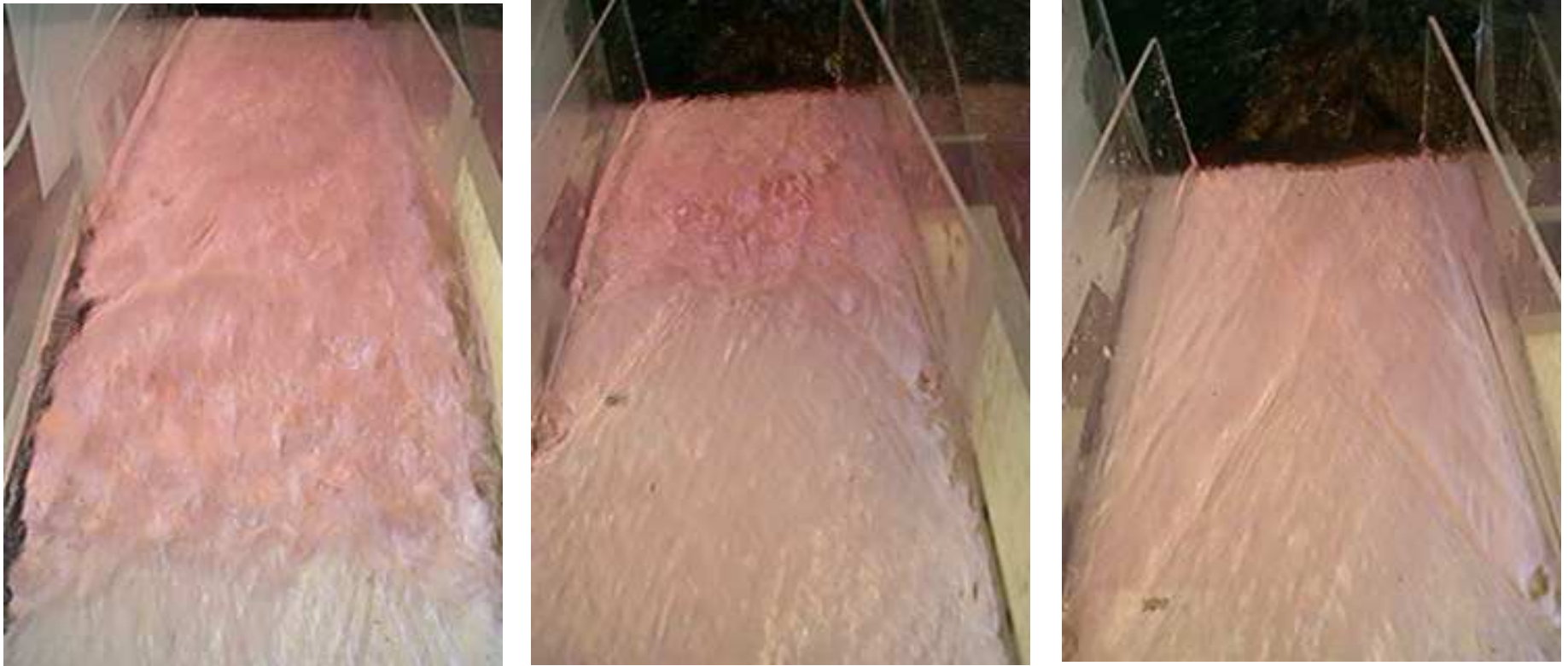
Fig. 4'. Multiple states: F_0 = 3.07 & B_c = 0.7 . Left to right: upstream steady shock (iii), reservoir state with "Mach stem" (iv), and oblique waves (i). Transitions induced by pushing flow.
